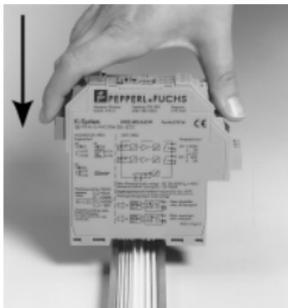
The K-system devices by Pepperl+Fuchs, including the universal signal conditioner KF\*\*-USC-1.D can be mounted on a 35 mm standard rail corresponding to DIN EN 50022. Simply snap on the devices **vertically**, never tipped or angled from the side.
