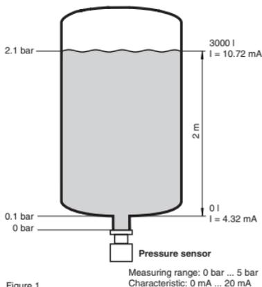
A pressure sensor with a measuring range of 5 bar and an output signal of 4 mA ... 20 mA is being used. With the full container the pressure sensor measures a pressure of 2.1 bar and outputs a current of 10.72 mA (figure 2).
