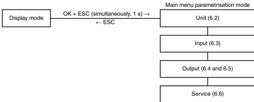
You can return to display mode from any point in the menu in parameterisation mode by pressing the ESC key (possibly multiple times). If you do not press any key for 10 minutes in parameterisation mode, the device automatically switches back into display mode.
