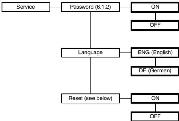
**Reset:** If *ON* is flashing and you press the *OK* key, all settings of the USC will be reset to the factory settings (see section 6.7). All entries which you have ever made in parameterisation mode will be lost.
