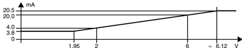
Input type 0 mV ... 60 mV, characteristic 2 V ... 10 V, start value 5 mV, end value 45 mV
