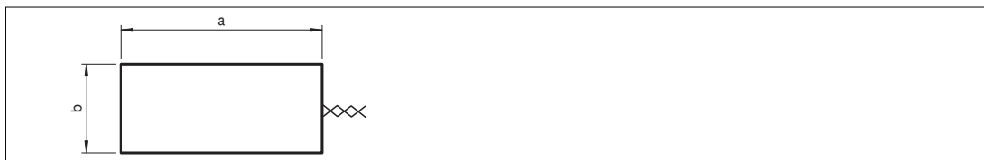
Figure 4.1 e.g.: a = 3 m; b = 1 m; U = 2 \times 3 \text{ m} + 2 \times 1 \text{ m} = 8 \text{ m} ; Number of windings = 4
