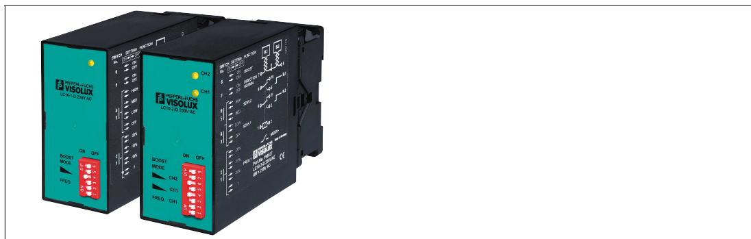
Figure 3.1 LC10-1 (left) and LC10-2 (right) loop detectors
