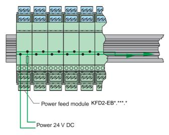
Wiring costs are significantly lower when supplying power via the Power Rail. It is also possible to take advantage of collective error messages and redundant power supply. A power failure is indicated via the power supply module signal contacts.
