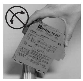
INCORRECT: Unit snapped on at an angle.
