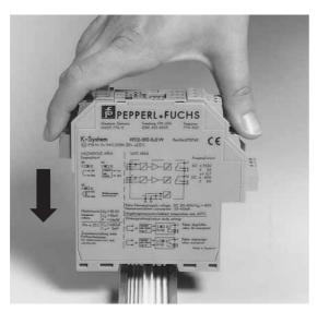
**CORRECT: Unit snapped on vertically.**
