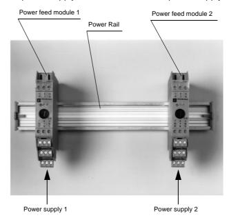
A redundant power supply to the Power Rail, with two supply modules, provides increased safety. If the fuse in one power supply module operates, the power supply is obtained via the second power supply module. Each power supply circuit is connected via its own Power Rail contact.
