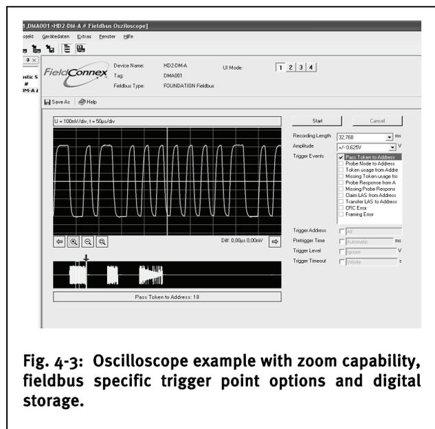
**Fig. 4-3: Oscilloscope example with zoom capability, fieldbus specific trigger point options and digital storage.**
