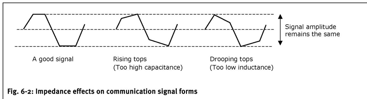
**Fig. 6-2: Impedance effects on communication signal forms**
