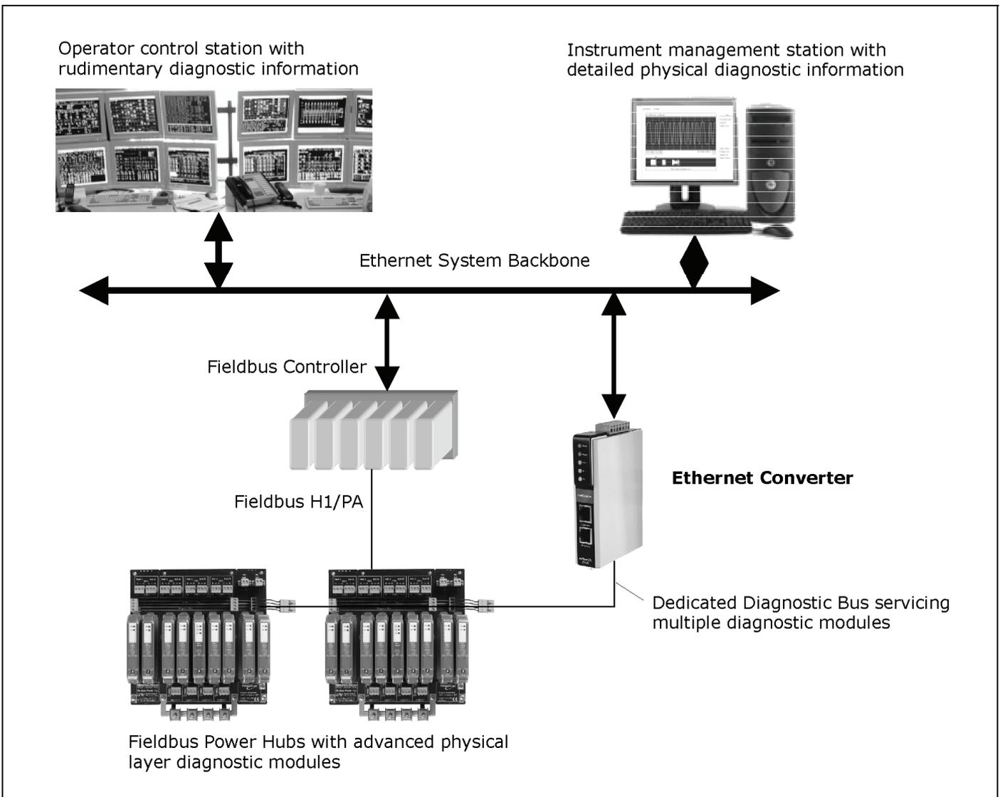
Fig. 5-1: Advanced physical layer diagnostic infrastructure
