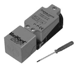
Speed monitors are inductive proximity switches in which both the damping status and the act of exceeding or falling short of a reference frequency is signalled. The reference frequency is adjusted via a built-in potentiometer. If the actual frequency  $f_{\text{act}}$  measured by the proximity switch is smaller than  $f_{\text{nom}}$ , the output is switched off. If the measured actual frequency  $f_{\text{act}}$  is greater than  $f_{\text{nom}}$ , the output is closed (switched on).
