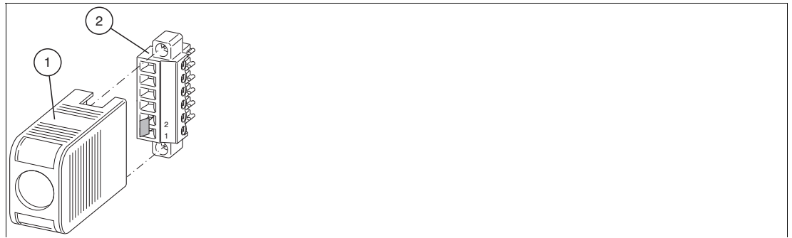
Figure 3.12 Cold junction for thermocouple measurements
