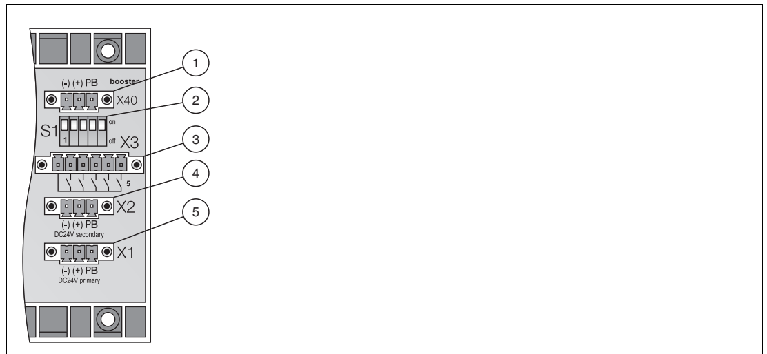
Figure 3.6 Connections on the right-hand side
