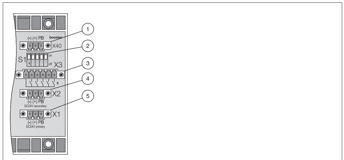
Figure 3.6 Connections on the right-hand side
