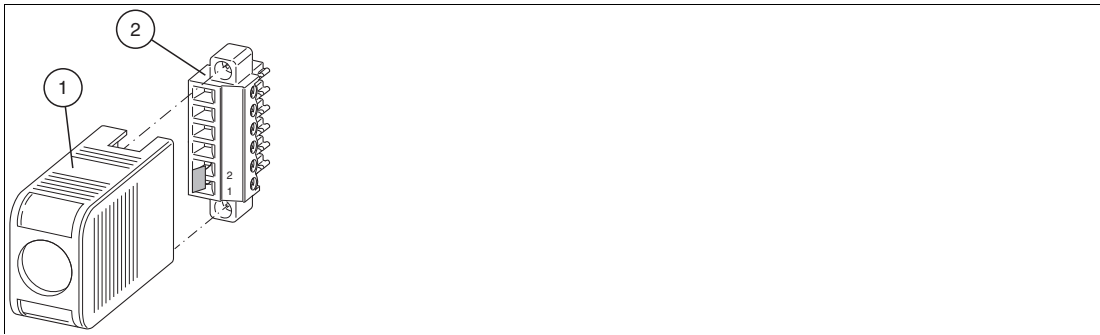
Figure 3.12 Cold junction for thermocouple measurements
