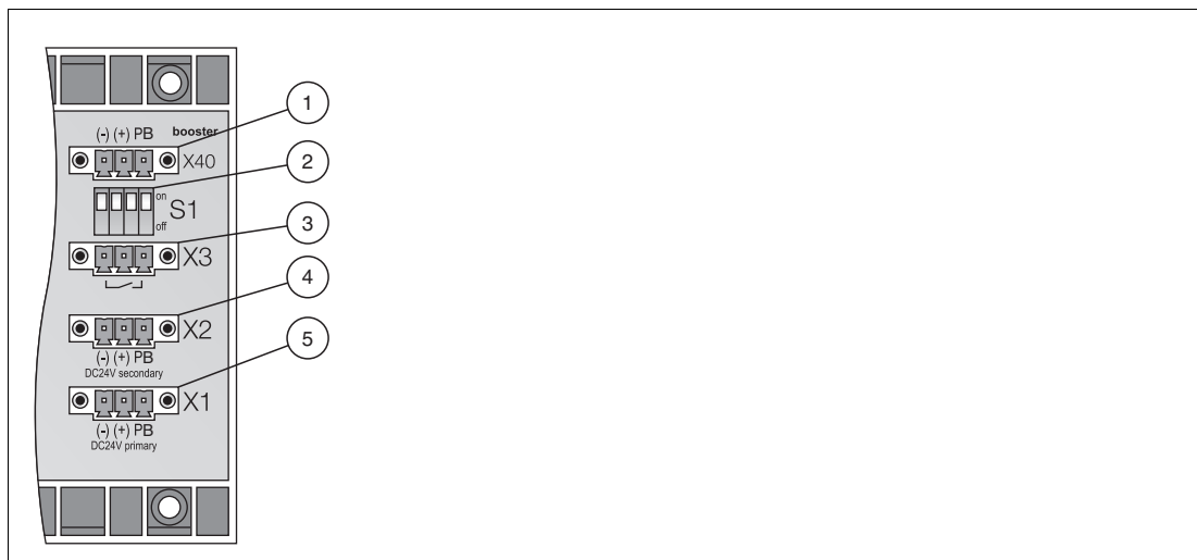
Figure 3.2 Connections on the right-hand side
