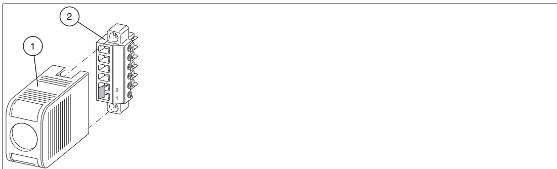
Figure 3.12 Cold junction for thermocouple measurements
