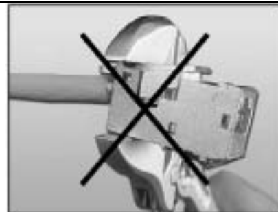
If the pliers are applied too far back, the loader may be displaced, damaging the ID connectors inside the module.
