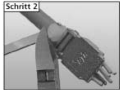
Fit a cable tie as strain relief and cut off the excess length.
