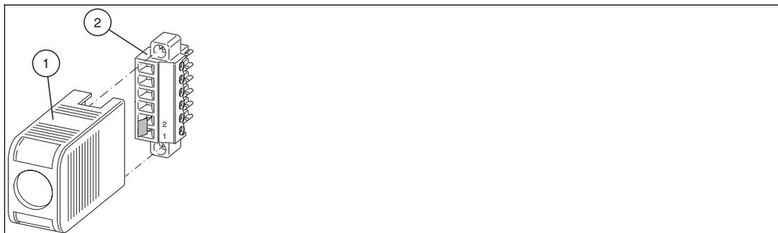
Figure 3.13 External cold junction for thermocouple measurements
