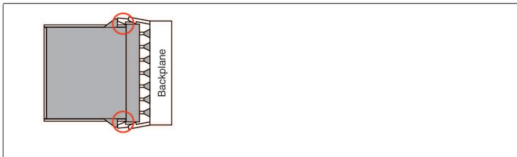
Figure 3.8 FB removal tool releases the second rear catch
