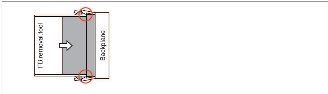
Figure 3.7 FB removal tool releases the first rear catch
