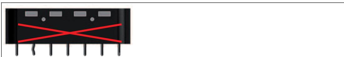
Figure 3.2 Bent connector pin
