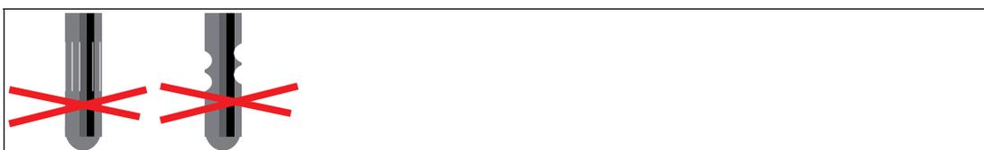
Figure 3.3 Damaged pins with nicks or scratches
