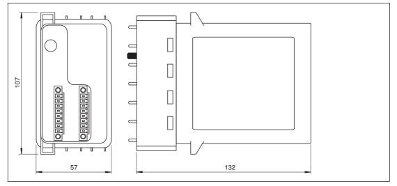
Figure 2.5 Dual-width module dimensions
