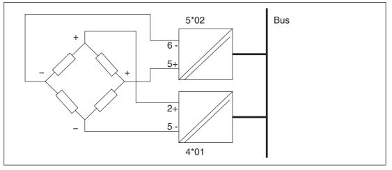
Figure 3.14 Example of a strain gauge bridge
