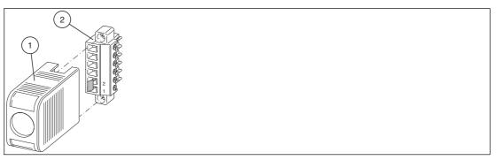
Figure 3.13 External cold junction for thermocouple measurements
