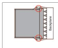
Figure 3.8 FB removal tool releases the second rear catch
