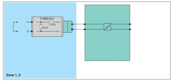
Figure 2.16 Block diagram of the F-NR2-Ex1 resistor network
