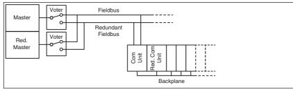
Figure 3.16 Extended media redundancy
