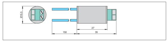
Figure 2.15 Dimensions of the F-NR2-Ex1 resistor network
