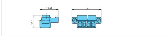
Figure 2.6 Screw terminal dimensions
