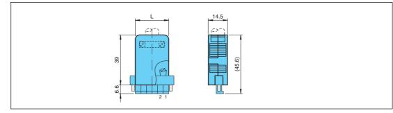
Figure 2.12 Dimensions of a cold junction with a protective cover
