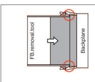
Figure 3.7 FB removal tool releases the first rear catch
