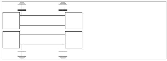
Figure 3.22 EMC filters in a network (simplified diagram)
