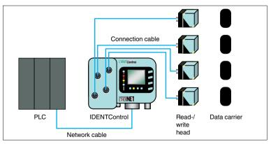
Figure 2.1: Installation of the hardware equipment
