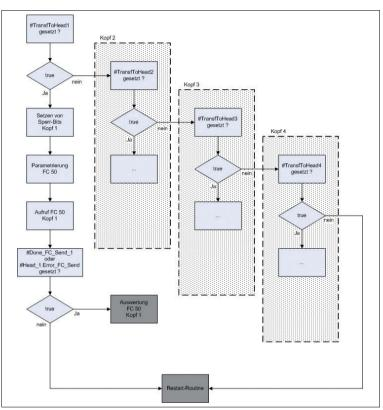
Figure 6.7: Program flow chart Command Execution Head 1
