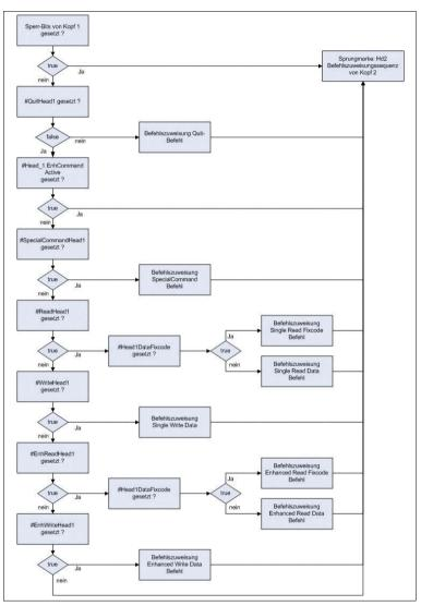
Figure 6.6: Program flow chart of Command Allocation of Head 1
