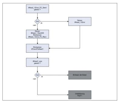
Figure 6.9: Program flow chart analysis FC 50 of head 1
