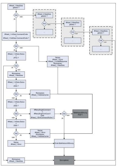
Figure 6.11: Program flow chart Analysis Input Data Fields
