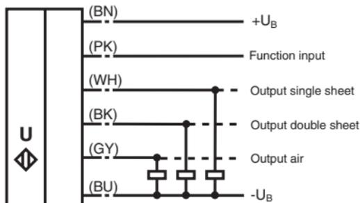
Bild 7.2: Electrical connection, versions ...-3E2 and ...-3E3
