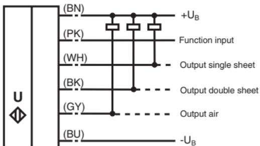
Bild 7.1: Electrical connection, versions ...-3E0 and ...-3E1
