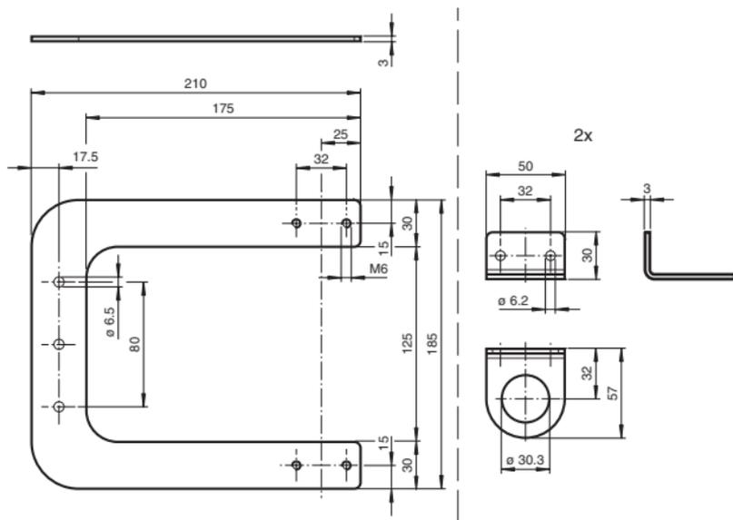
Bild 8.1: Dimensions - Installation device MH-UDB-02
