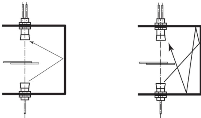
Bild 4.3: Indirect sound propagation due to reflection on the mounting bracket
