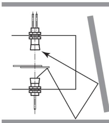
Bild 4.4: Indirect sound propagation due to reflection on plant components
