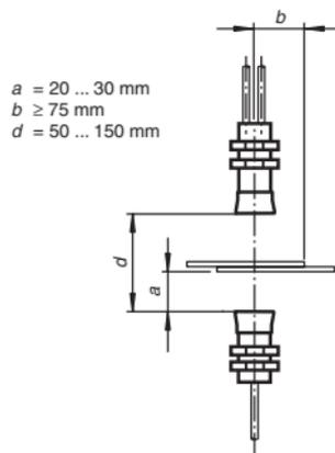
Bild 4.1: Recommended separations and angular adjustments
