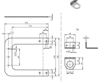
Bild 8.1: Dimensions - Installation device MH-UDB-02
