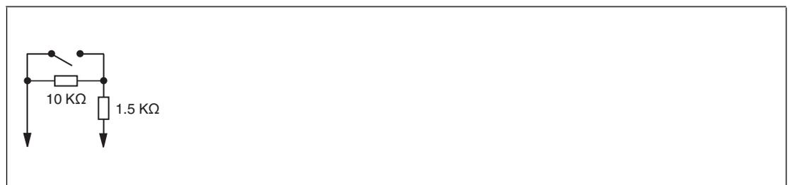
Figure 8.28 Resistor network for line fault detection
