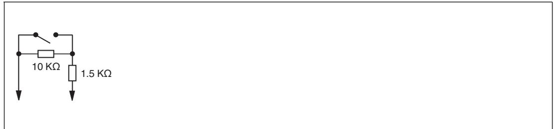
Figure 8.8 Resistor network for line fault detection
