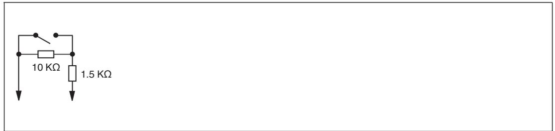
Figure 8.89 Resistor network for line fault detection
