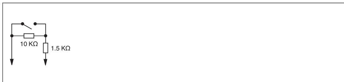
Figure 8.17 Resistor network for line fault detection
