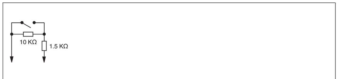
Figure 8.5 Resistor network for line fault detection
