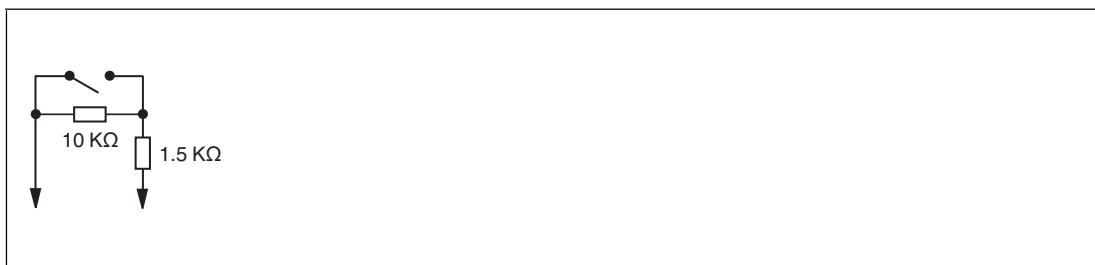
Figure 8.21 Resistor network for line fault detection
