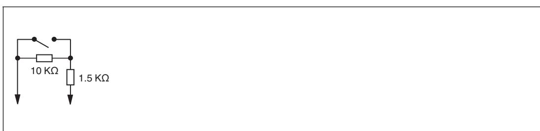
Figure 8.13 Resistor network for line fault detection
