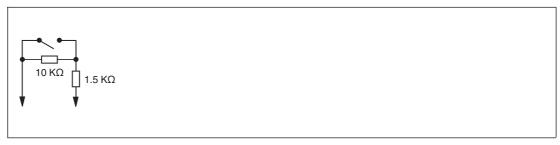
Figure 8.5 Resistor network for line fault detection
