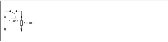
Figure 8.17 Resistor network for line fault detection
