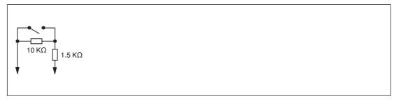
Figure 8.21 Resistor network for line fault detection
