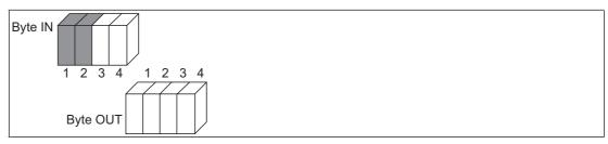
Figure 3.4 Universal module 4I4O populated with 2 bytes input data
