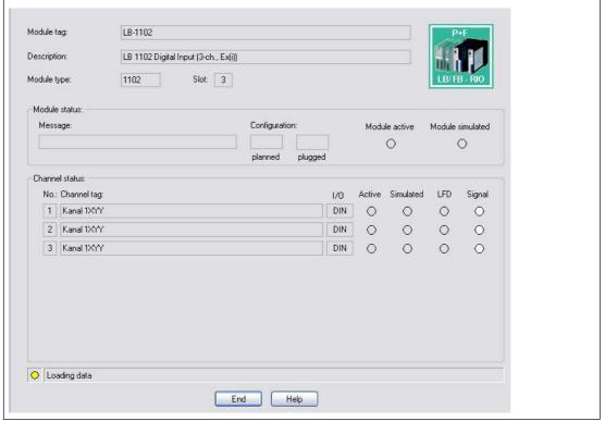
Figure 7.7 Show Measured Value window for digital modules
