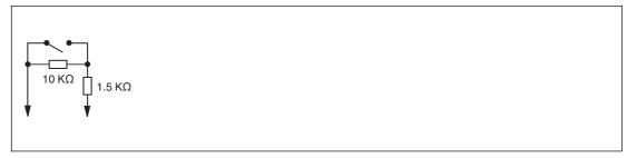
Figure 8.2 Resistor network for line fault detection
