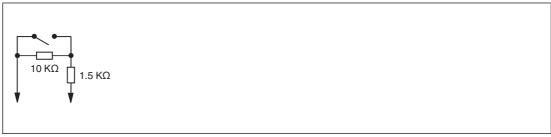
Figure 8.28 Resistor network for line fault detection
