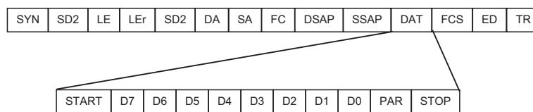
Figure 2.3: Structure of the Profibus telegram
