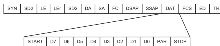
Figure 2.3: Structure of the Profibus telegram
