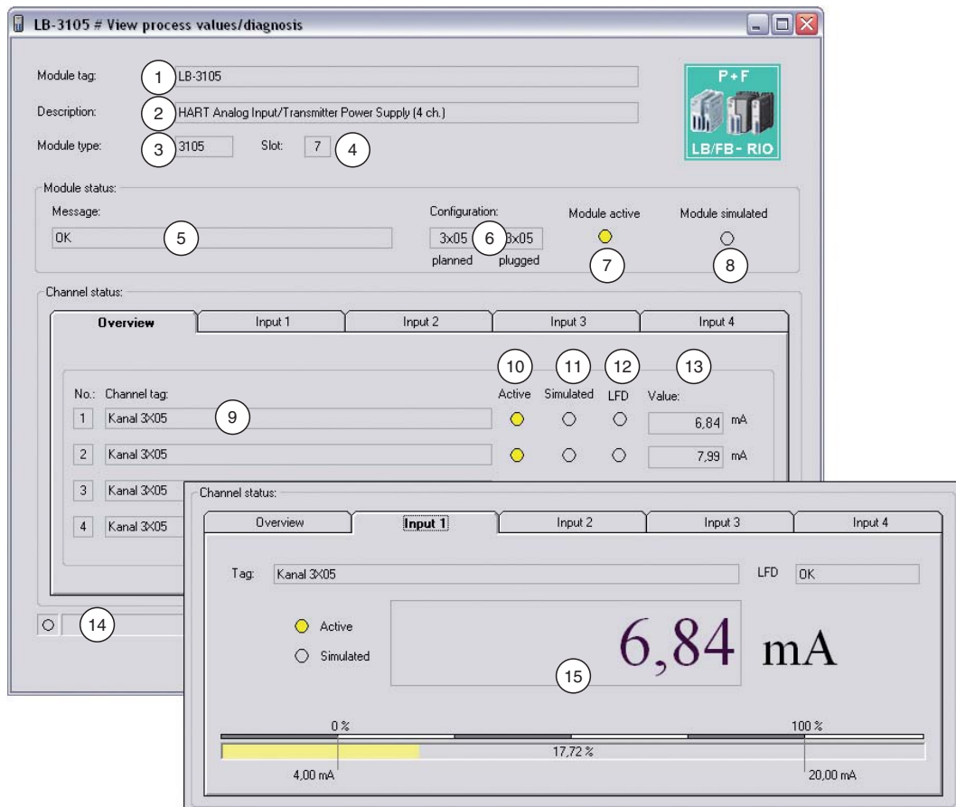
Figure 6.5: View process values/diagnosis window
