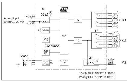
Figure 2: Block diagram
