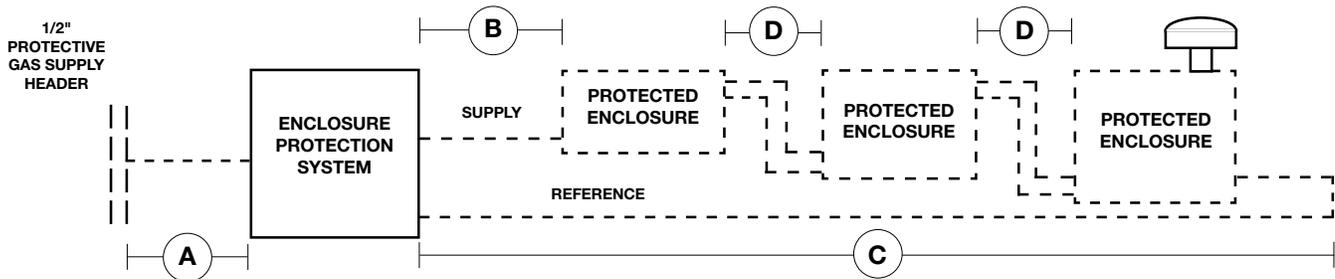
**\*NOTE:** Tube and pipe sizes are trade sizes and are not equal in inside diameter. DO NOT substitute tube for pipe with same trade size.
