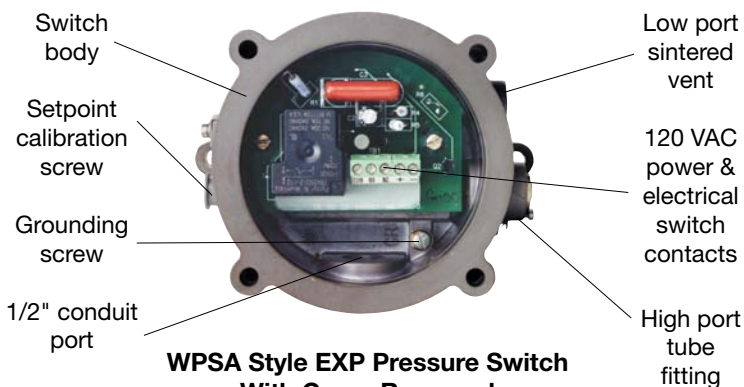
WPS Style EXP Pressure Switch With Cover Removed
