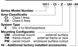
FM & PM confi uration mounting plates include four (4) 1/4" mounting holes at each corner, on 5/16" centers.
