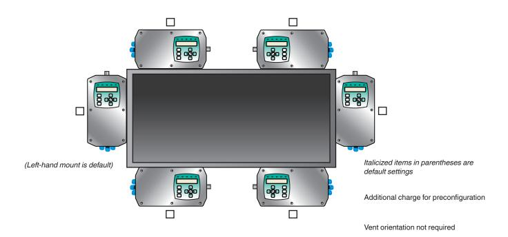
When rotating the UIC display in the housing, always torque adjacent screws at 0.46 N-m (4 in-lb).
