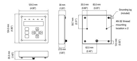
The user interface can be mounted either inside or outside the pressurized enclosure using the dimensions in the two previous drawings above.
