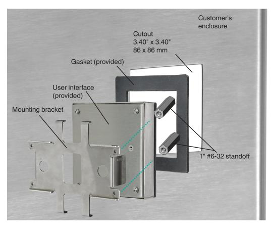
Use a crisscross pattern to tighten the screws for the UIC bracket. Tighten bolts 0.4 N-m (3 to 4 in-lb). For a good seal, ensure that the bracket bottoms out on the enclosure.
