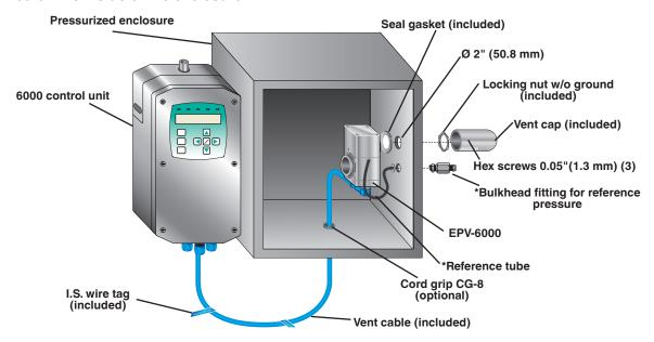
$\frac{\mathbf{O}}{\mathbf{I}}$  Vent is not gravity-sensitive and can be installed in any orientation.
