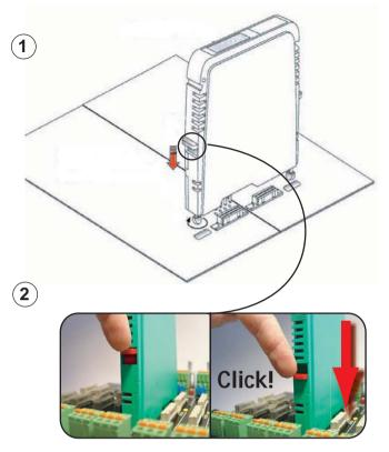
The new module has been installed.
