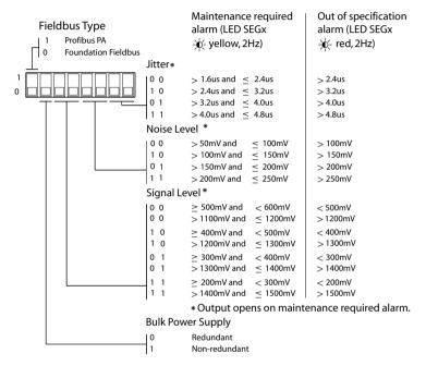
The voltage-free relay output opens if a value violates the preset maintenance required limit. (see chapter 6.1).
