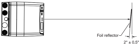
Figure 5.6: Foil reflector arrangement (top view of VDM)
