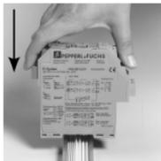
The devices of the K-system from Pepperl+Fuchs and thus also the Universal Transmitter Power-Supply KF\*\*-CRG2-(Ex)1.D can be mounted on a 35 mm DIN mounting rail according to DIN EN 60715. The devices must be snapped onto the rail **vertically**, and never slanted or tipped to the side.
