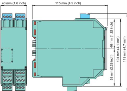
Dimensions of the device in mm
