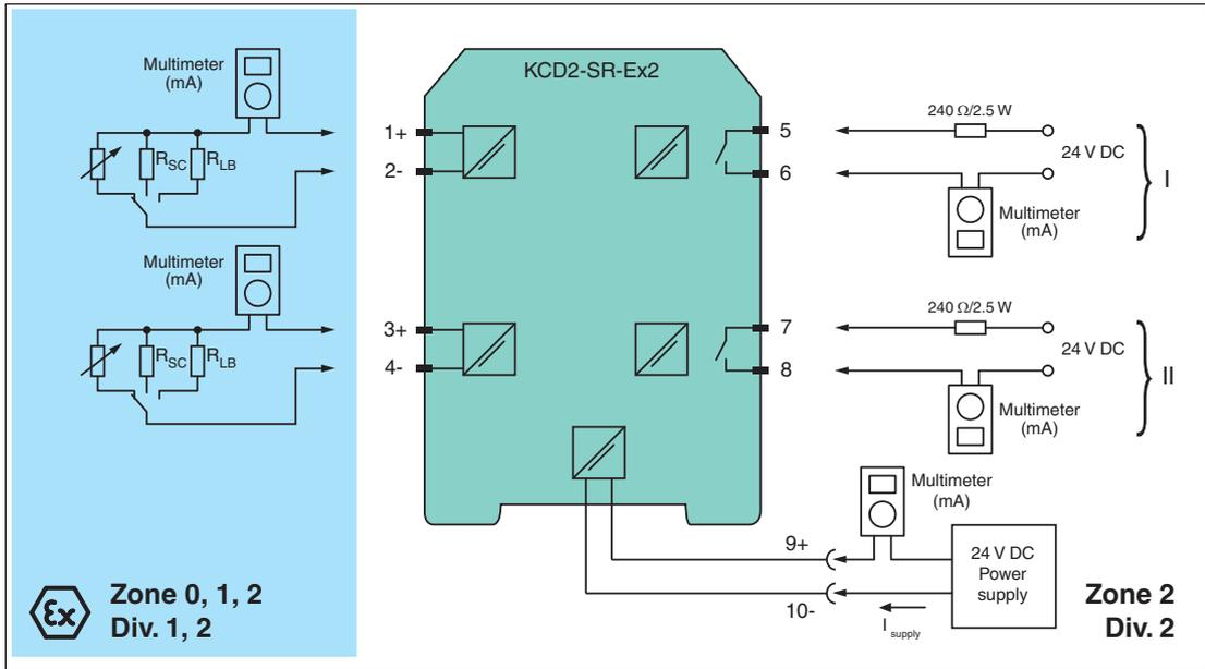
Figure 5.2 Proof test set-up for KCD2-SR-(Ex)2(.SP)
