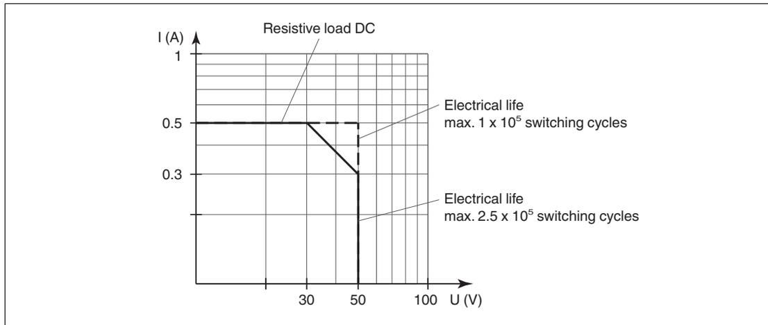
Figure 3.1 Maximum switching power of HiC282\*
