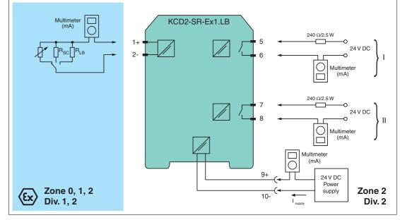
Figure 5.1 Proof test set-up for KCD2-SR-(Ex)1.LB(.SP)
