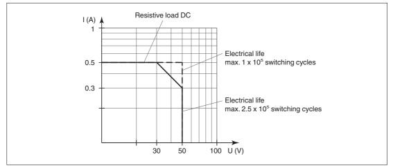
Figure 3.1 Maximum switching power of HiC282\*
