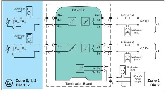
Figure 5.3 Proof test set-up for HiC2821, HiC2822
