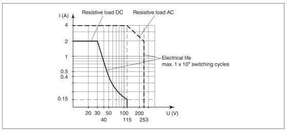
Figure 3.2 Maximum switching power of KCD2-SR-(Ex)\*(.LB)(.SP)
