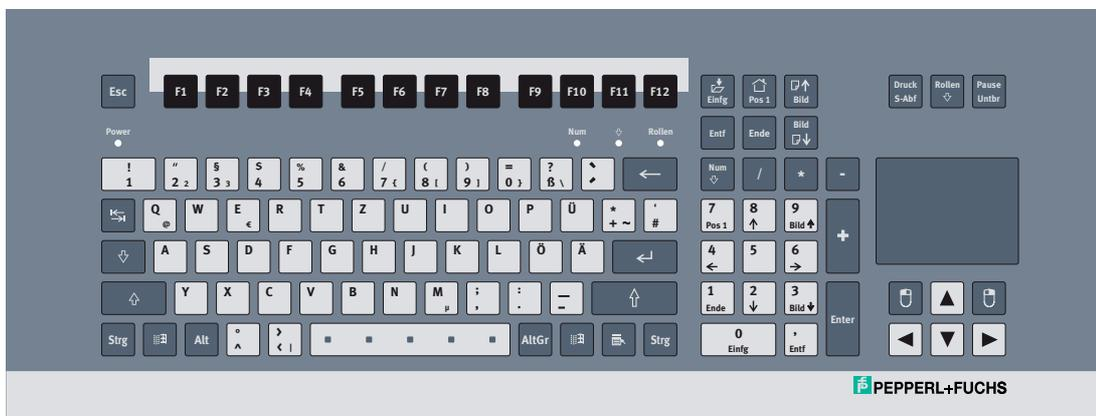
The keyboard foil is manufactured from a biaxially aligned polyester-based material and therefore has a greater resistance to solvents. The foil is stronger and more durable than other standard foils used on keyboards and front panels, such as polycarbonate and PVC.
