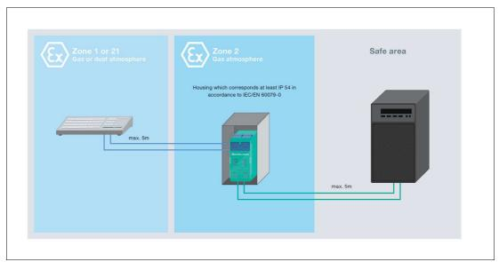
Figure 3.1 Installation requirements for the barrier in Zone 2 (gas) option 1
