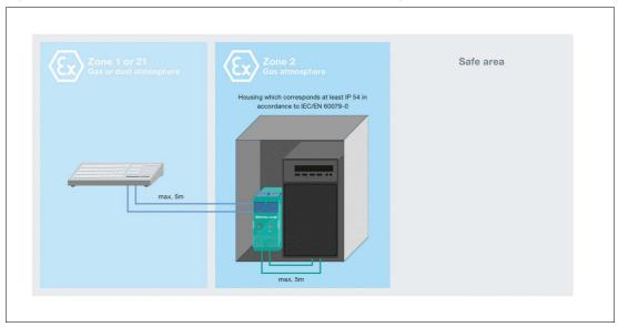
Figure 3.2 Installation requirements for the barrier in Zone 2 (gas) option 2
