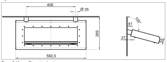
Figure 3.16 Dimensiondrawing
