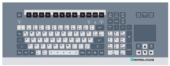
The keyboard foil is manufactured from a biaxially alignned polyester-based material and therefore has a greater resistance to solvents. The foil is stronger and more durabe than other standard foils used on keyboards and front panels, such as polycarbonate and PVC.
