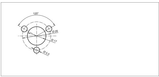
Figure 3.17 Drilling pattern for the wall
