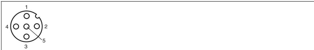
Pin assignment of the M12 socket for RS 232
