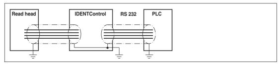
The cable shielding is used to discharge electromagnetic interference. When shielding a cable, you must connect both sides of the shield to ground with low resistance and low inductance.
