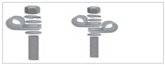
7. Attach the PE cable. Depending on the version of the keyboard there are one or two cables.
