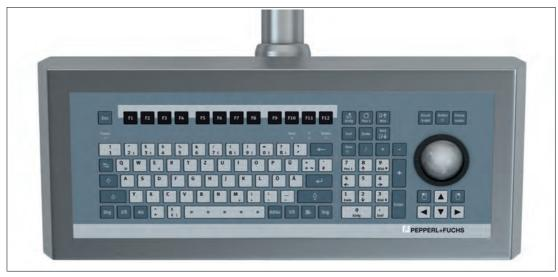
Figure 2.7 Keyboard with optical trackball
