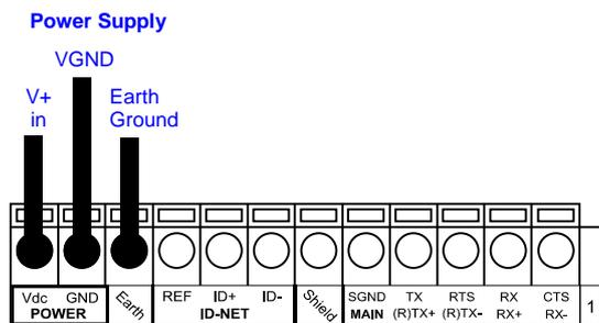
Figure 18 - Power Supply Connections
