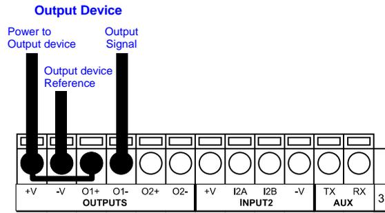
Figure 36 - Open Emitter Output Using VB14N Power
