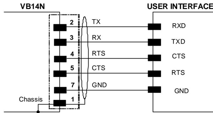
Figure 42 – RS232 Main Interface Connections Using Hardware Handshaking
