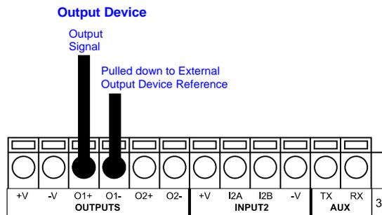
Figure 39 - Open Collector Output Using External Power
