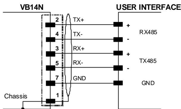
Figure 44 - RS485 Full-duplex Connections
