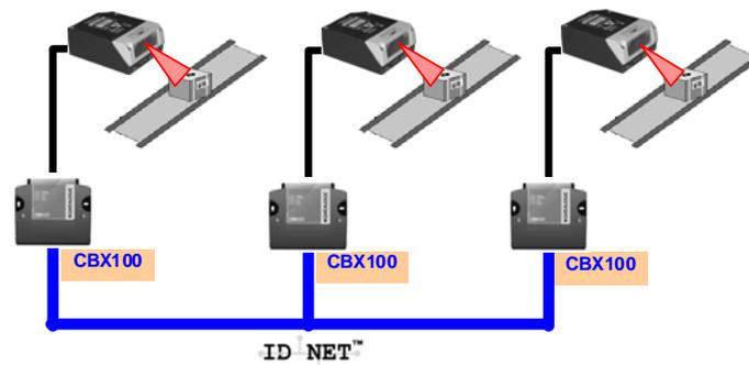
ID-NET™ interface allows connection of scanners reading objects placed on independent conveyors. All scanners are typically located far away from each other and they use a dedicated presence sensor.
