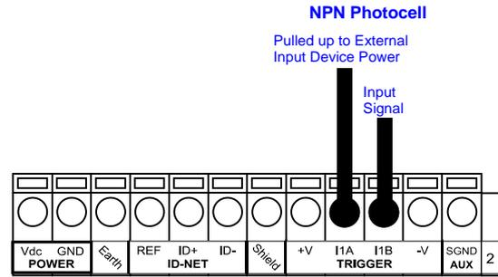
Figure 33 - NPN External Trigger Using External Power
