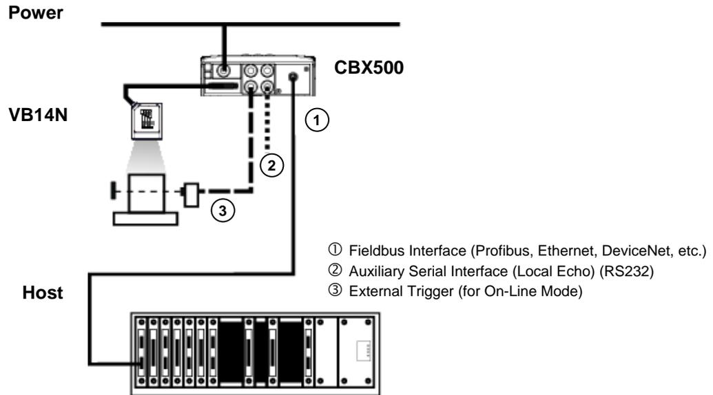
Figure 64 – Fieldbus Interface Point-to-Point Layout
