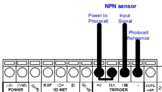
Figure 31 - NPN External Trigger Using VB14N Power
