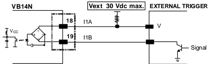
Figure 56 - NPN External Trigger Using External Power
