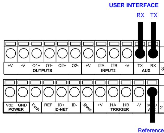
Figure 29 - RS232 Auxiliary Interface Connections
