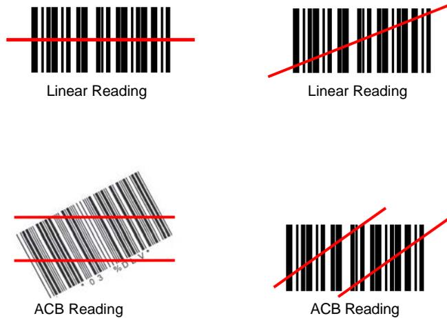
ACB reads two fragments of a label containing a start or a stop character and a number of digits, and puts them together to build the complete label.
