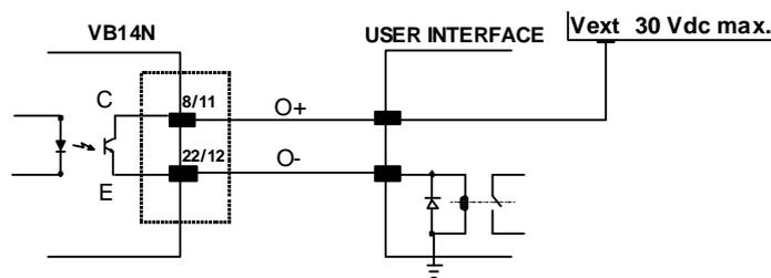
Figure 61 - Open Emitter Output Connections
