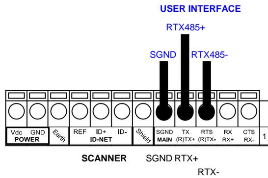
**Figure 23 - RS485 Half-duplex Connections**
