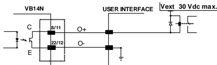
Figure 62 - Open Collector Output Connections
