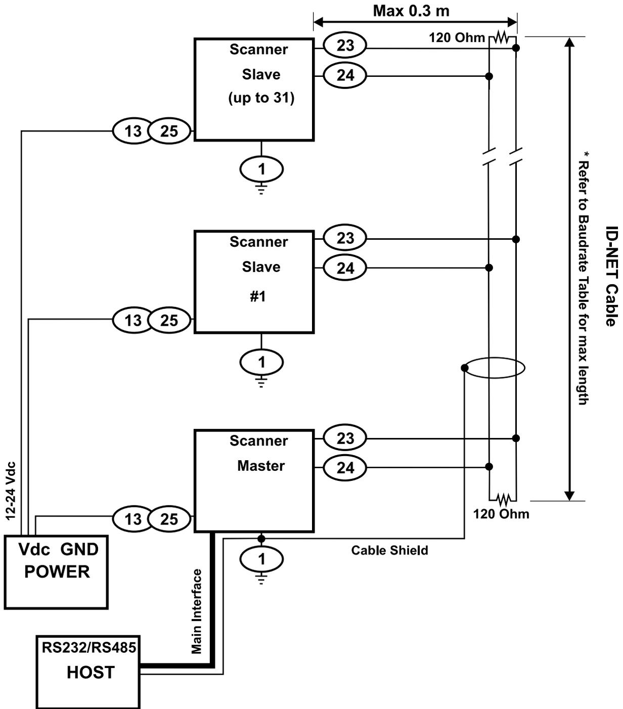
Figure 50 – ID-NET™ Network Connections with Common Power Star Network
