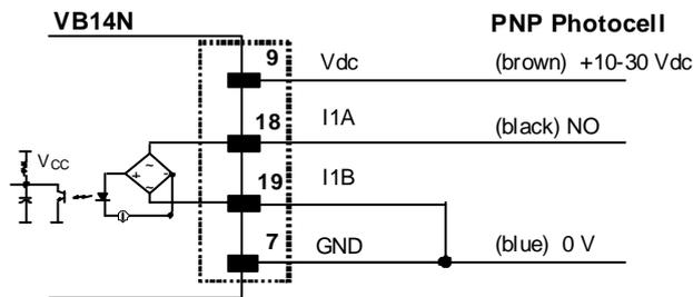
Figure 52 - Photocell (PNP) External Trigger Using VB14N Power
