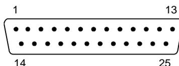
Figure 40 - 25-pin Male D-sub Connector
