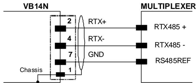
**Figure 46 - RS485 Half-duplex Connections**
