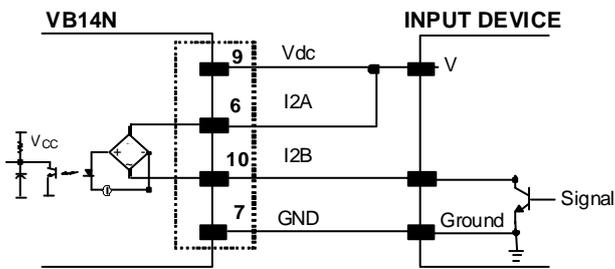
Figure 58 - NPN Input 2 Using VB14N Power
