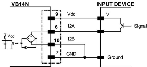
Figure 57 - PNP Input 2 Using VB14N Power
