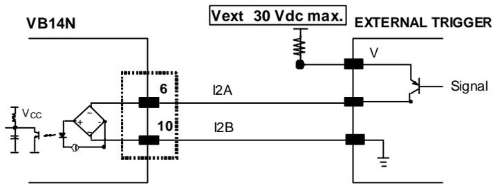
Figure 59 - PNP Input 2 Using External Power
