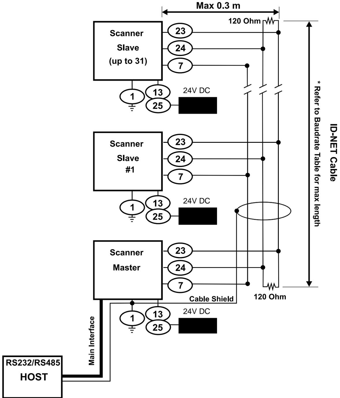
Figure 48 – ID-NET™ Network Connections with isolated power blocks
