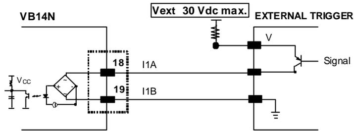
Figure 55 - PNP External Trigger Using External Power
