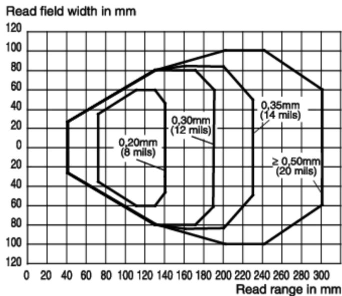
**NOTE:** (0,0) is the center of the laser beam output window.
