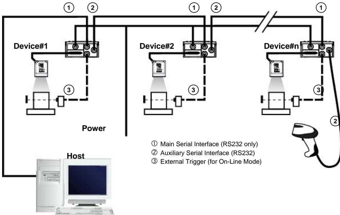
Figure 65 – Pass-Through Layout
