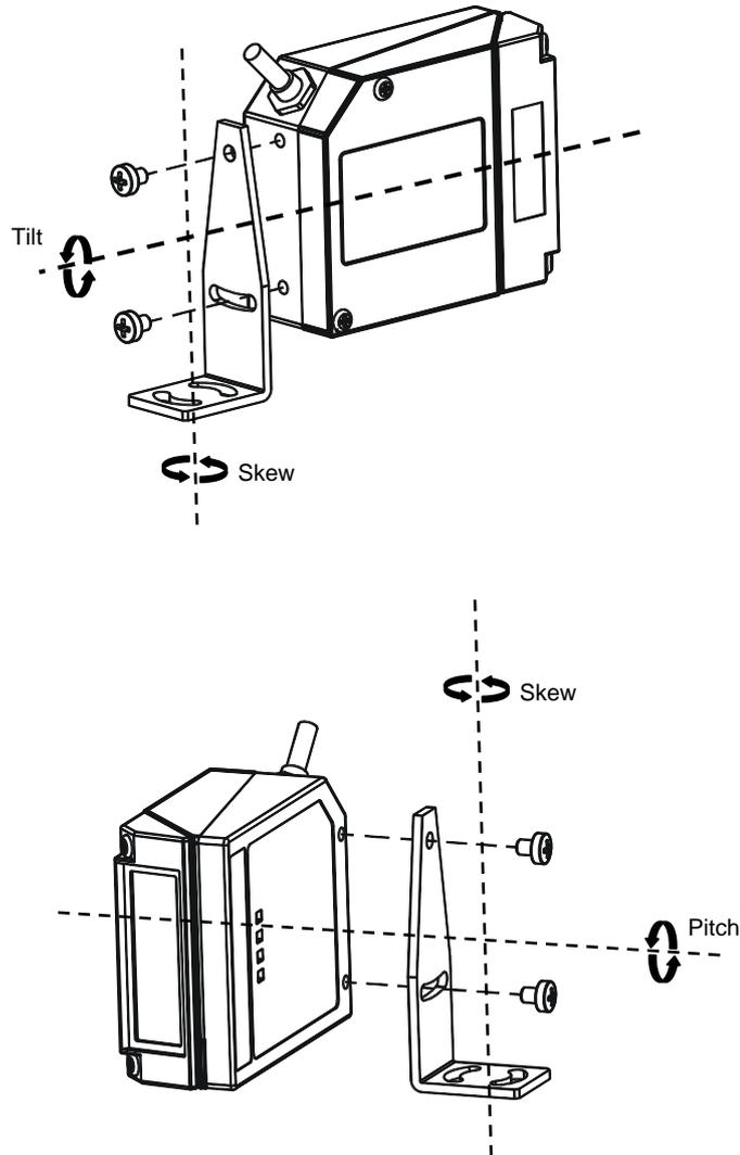
Figure 13 – Positioning with Mounting Bracket
