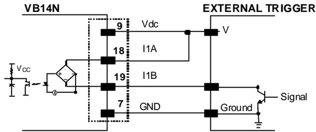
Figure 54 - NPN External Trigger using VB14N Power
