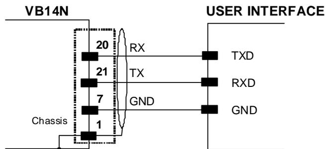
Figure 51 - RS232 Auxiliary Interface Connections
