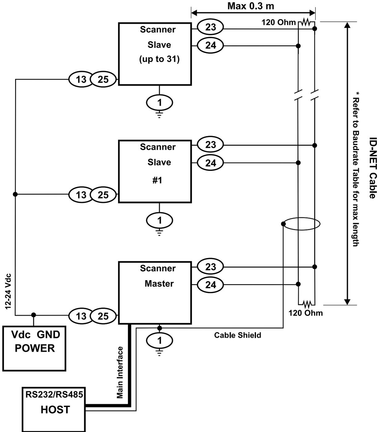
Figure 49 - ID-NET™ Network Connections with Common Power Branch Network
