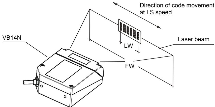
Figure 73 - "Picket-Fence" Scanning Mode
