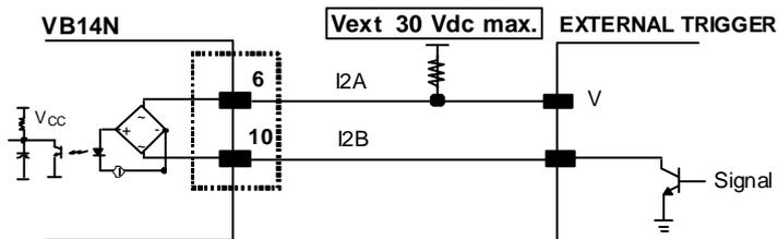
Figure 60 - NPN Input 2 Using External Power
