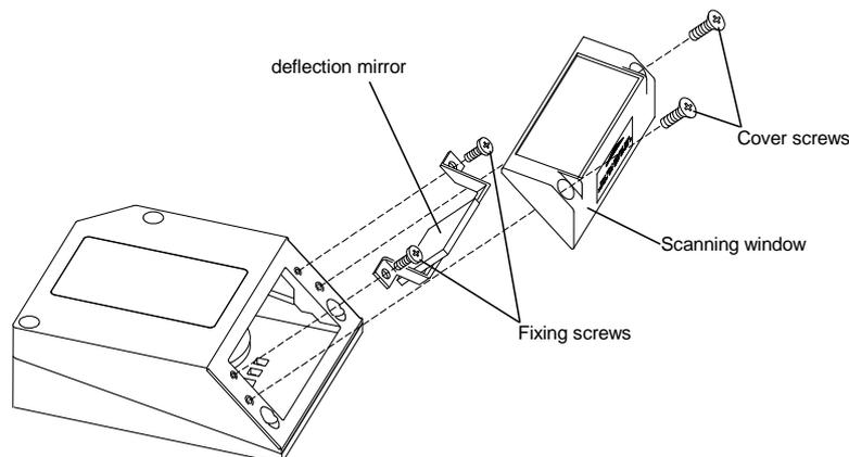
**Figure 14 - Installation of the Deflection Mirror**
