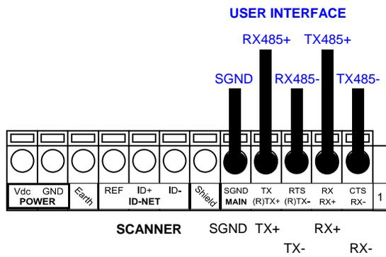
Figure 21 - RS485 Full-duplex Connections
