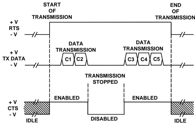
Figure 20 - RS232 Control Signals
