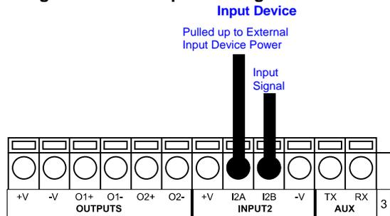
**Figure 35 - NPN Input 2 Using External Power**
