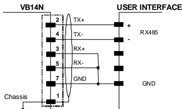
Figure 45 - RS485 Full-duplex Connections using Only TX Signals
