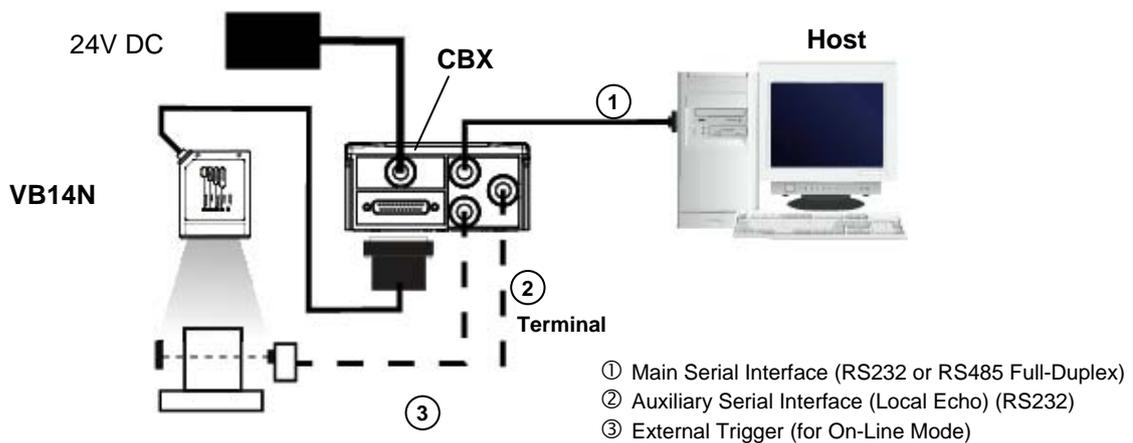
Figure 63 – Serial Interface Point-to-Point Layout
