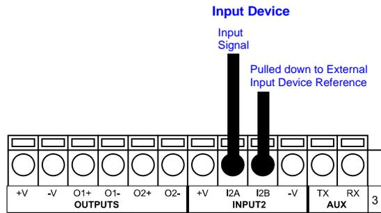
**Figure 34 - PNP Input 2 Using External Power**
