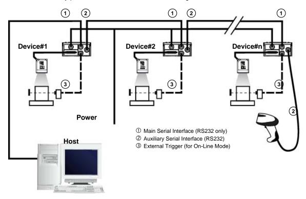
Figure 65 - Pass-Through Layout
