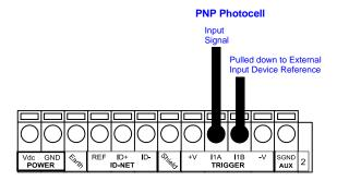
Figure 32 - PNP External Trigger Using External Power
