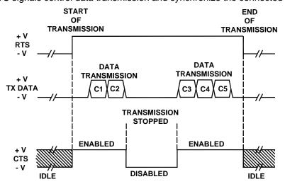
Figure 43 - RS232 Control Signals
