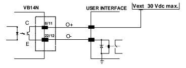
Figure 61 - Open Emitter Output Connections
