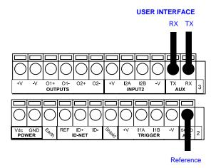
Figure 29 - RS232 Auxiliary Interface Connections
