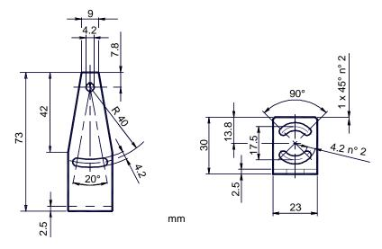
Figure 12 - Mounting Bracket Overall Dimensions
