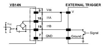
Figure 54 - NPN External Trigger using VB14N Power
