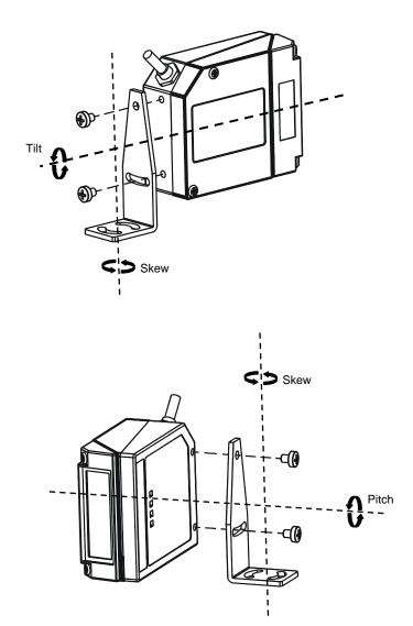
Figure 13 – Positioning with Mounting Bracket
