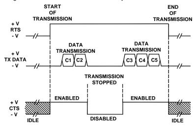
Figure 20 - RS232 Control Signals
