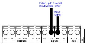
Figure 35 - NPN Input 2 Using External Power
