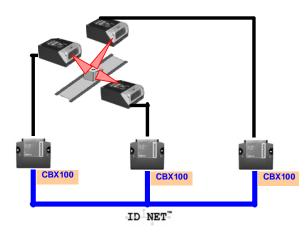
ID-NET™ interface allows local connection of multiple scanners reading different sides of the same target. All scanners share a single presence sensor and activate/deactivate simultaneously.
