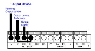
Figure 37 - Open Collector Output Using VB14N Power
