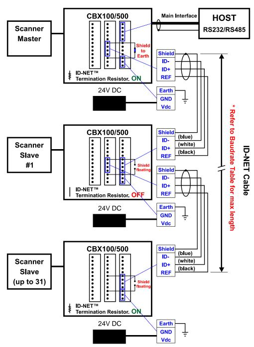
Figure 25 – ID-NET™ Network Connections with isolated power blocks
