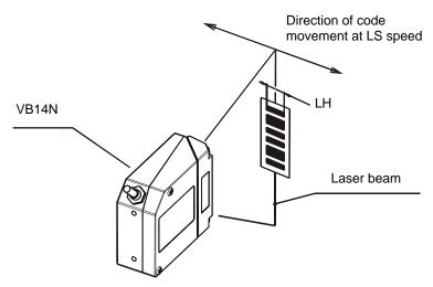
Figure 72 - "Step-Ladder" Scanning Mode
