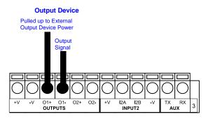
Figure 38 - Open Emitter Output Using External Power
