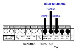
Figure 22 - RS485 Full-duplex Connections using Only TX Signals
