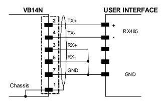
Figure 45 - RS485 Full-duplex Connections using Only TX Signals
