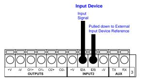
Figure 34 - PNP Input 2 Using External Power Input Device
