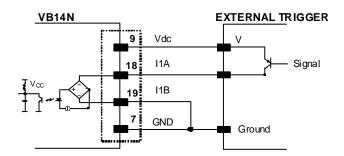
Figure 53 - PNP External Trigger Using VB14N Power
