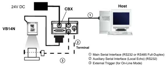
Figure 63 - Serial Interface Point-to-Point Layout
