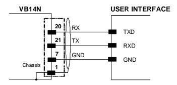
Figure 51 - RS232 Auxiliary Interface Connections
