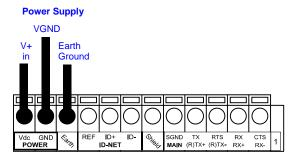
Figure 18 - Power Supply Connections
