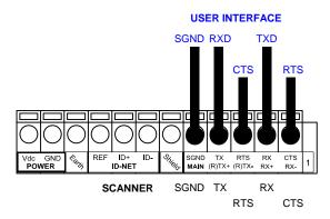
Figure 19 – RS232 Main Interface Connections Using Hardware Handshaking
