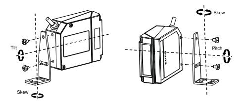
Figure 3 - Positioning with Mounting Bracket
