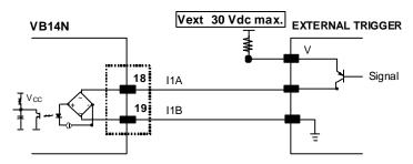
Figure 55 - PNP External Trigger Using External Power
