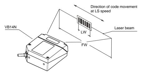
Figure 73 - "Picket-Fence" Scanning Mode
