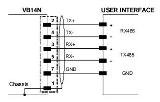
Figure 44 - RS485 Full-duplex Connections
