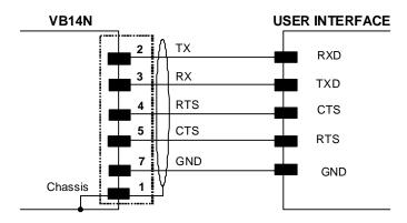
Figure 42 - RS232 Main Interface Connections Using Hardware Handshaking
