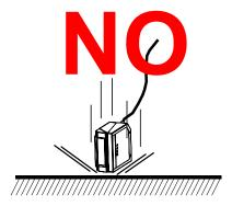
• do not fine tune the positioning by striking the scanner or bracket.
