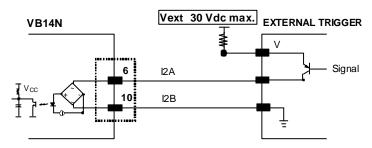
Figure 59 - PNP Input 2 Using External Power
