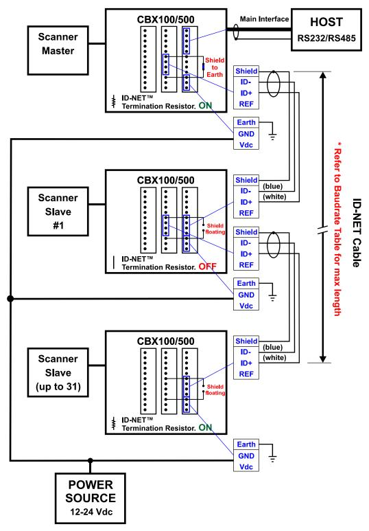
Figure 26 - ID-NET™ Network Connections with Common Power Branch Network
