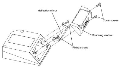
Figure 14 - Installation of the Deflection Mirror
