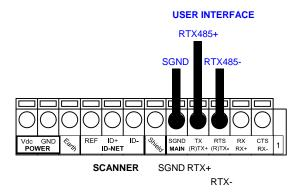
Figure 23 - RS485 Half-duplex Connections
