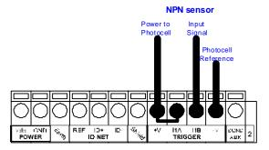
Figure 31 - NPN External Trigger Using VB14N Power
