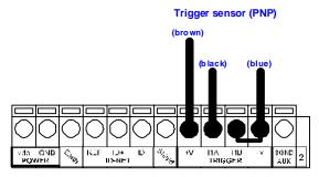
Figure 30 - Trigger sensor (PNP) External Trigger Using VB14N Power
