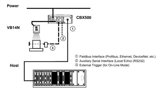
Figure 64 - Fieldbus Interface Point-to-Point Layout
