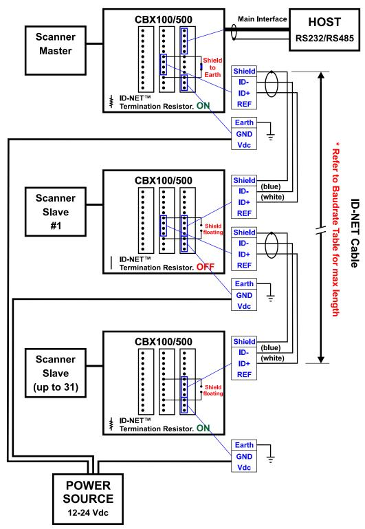
Figure 27 – ID-NET™ Network Connections with Common Power Star Network
