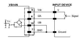
Figure 57 - PNP Input 2 Using VB14N Power
