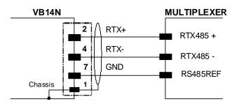
Figure 46 - RS485 Half-duplex Connections
