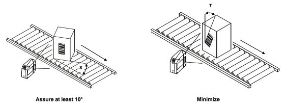
Figure 4 – Skew and Tilt Angles
