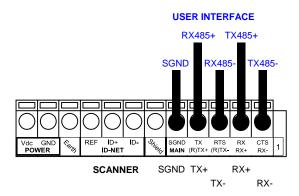
Figure 21 - RS485 Full-duplex Connections
