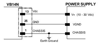
Figure 41 - Power Supply Connections
