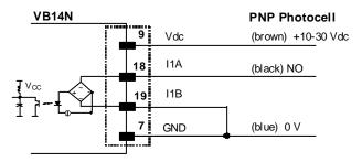
Figure 52 - Photocell (PNP) External Trigger Using VB14N Power
