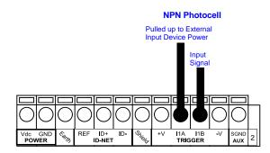
Figure 33 - NPN External Trigger Using External Power
