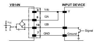
Figure 58 - NPN Input 2 Using VB14N Power
