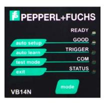
The colors and meaning of the five LEDs are illustrated in the following table:
