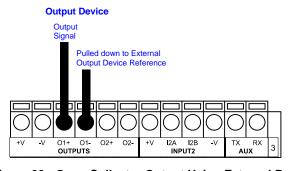
Figure 39 - Open Collector Output Using External Power
