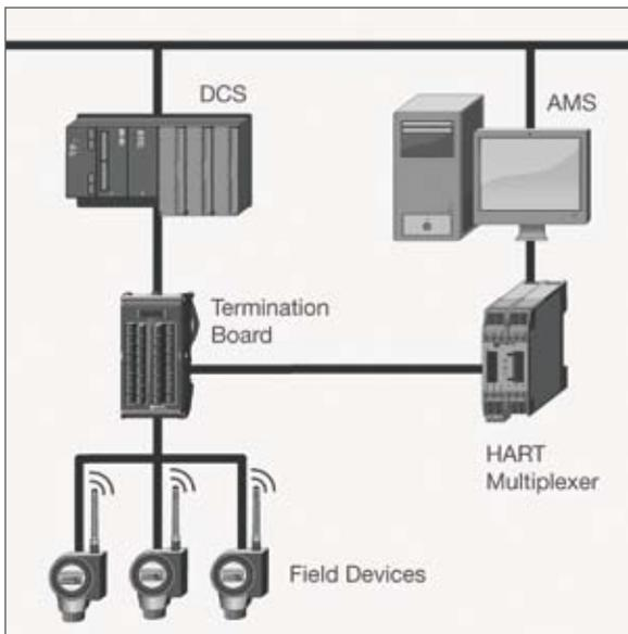
**Fig. 4: Structure of Conventional HART infrastructure**
