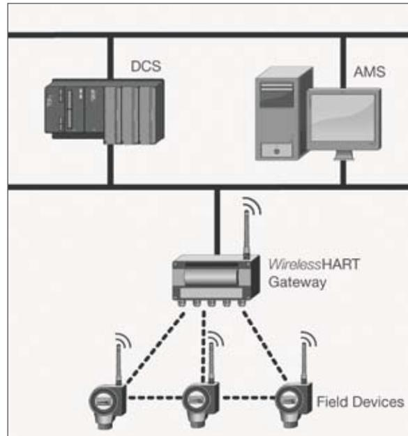
**Fig. 5: Structure new *WirelessHART* infrastructure**
