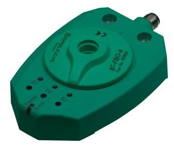
The PMI360DV-F130-IU2E2-V15 has an analog output for the indication of angular positions. For high resistance loads (>3.3 kΩ), the angular position will output a voltage value 0 ... 10 V DC and for low resistance loads (<400 Ω), a current value 4 ... 20 mA. In addition, the PMI360DV-F130-IU2E2-V15 has two switching outputs that can be programmed independently of one another and that can be used to mark two important positions (e.g., start and stop position).
