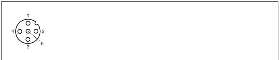
Figure 2.3 Slave connection (M12 socket)
