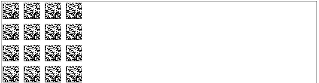
Figure 8.14 The code card assigns the orientation 180° to the read head.
