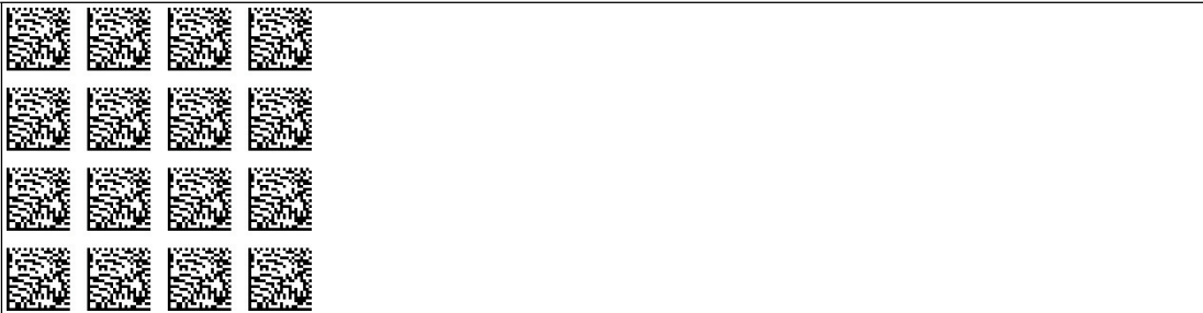
Figure 8.12 The code card assigns a position data resolution of 0.1 mm / 1 mm / 10 mm to the reading head.
