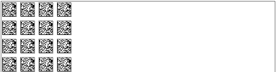
Figure 8.15 The code card automatically assigns the orientation 0° or 180° to the read head.
