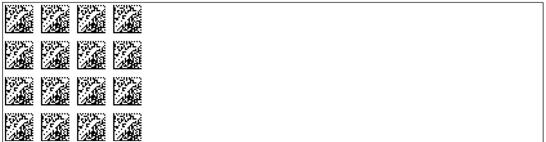
Figure 8.2 The code card "STORE" stores the modified parameterization in the non-volatile memory of the reading head and terminates external parameterization operating mode.
