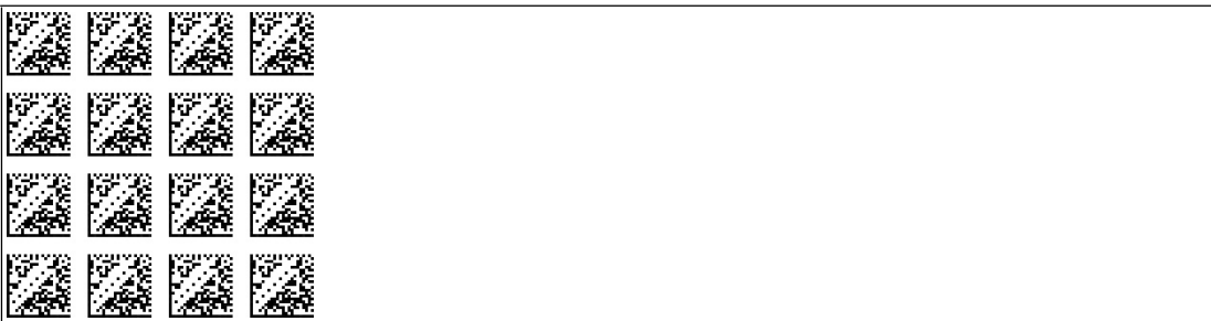
Figure 8.4 The "USE" code card takes over the set configuration volatile in the read head working memory and terminates the external parameterization operating mode. The read head then operates with this configuration. However, if the read head is switched off and on again, the configuration is lost and the read head operates with the last valid configuration that was saved. This function is used primarily for test purposes.
