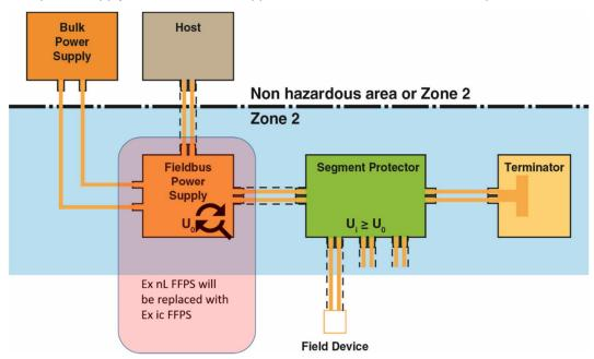
It is permitted to replace the failed fieldbus power supply for both scenarios. They can be replaced and the loops will remain Ex nL, if the user has conducted and documented the following action:
