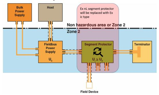
It is permitted to replace the segment protector. Type of protection for the loops remain Ex nL, if the user has conducted and documented the following actions:
