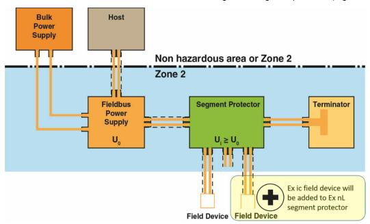
Ex ic-rated field devices can be added to the topology and the type of protection remains Ex nL with the following user actions:
