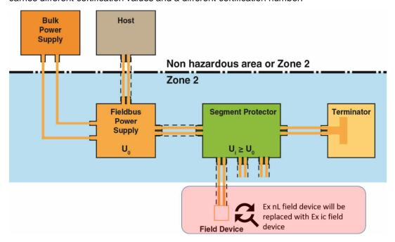
It is permitted to replace the field instrument. The loop remains Ex nL, if the user has conducted and documented the following actions:
