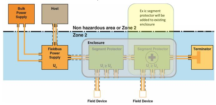
Ex ic rated segment protectors can be added to the topology and the type of protection remains Ex nL with the following user actions:
