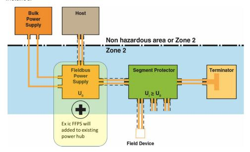
Ex ic rated power supply modules can be added to the topology and the type of protection remains Ex nL with the following user actions:
