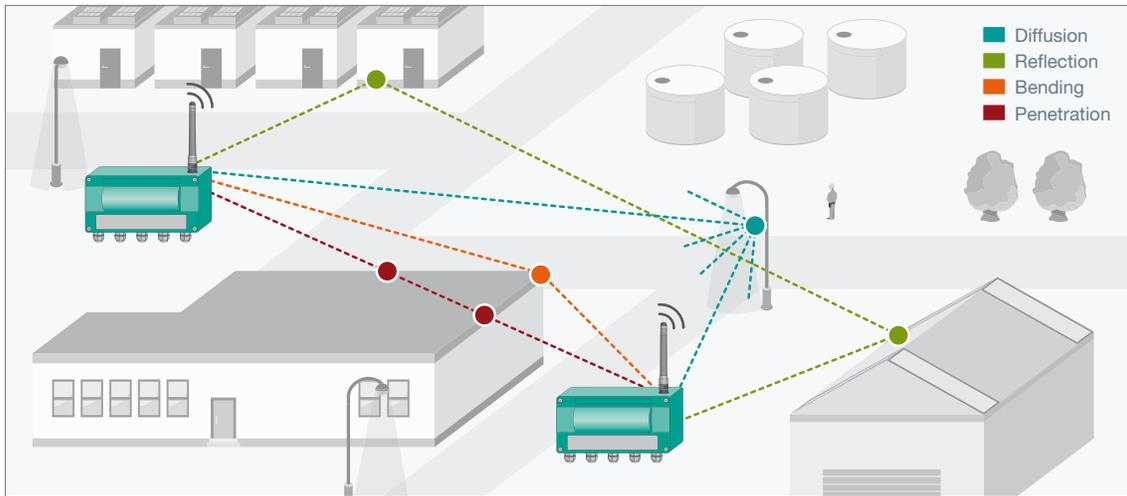
Figure 6: Diffusion, reflection, bending, and penetration of obstacles
