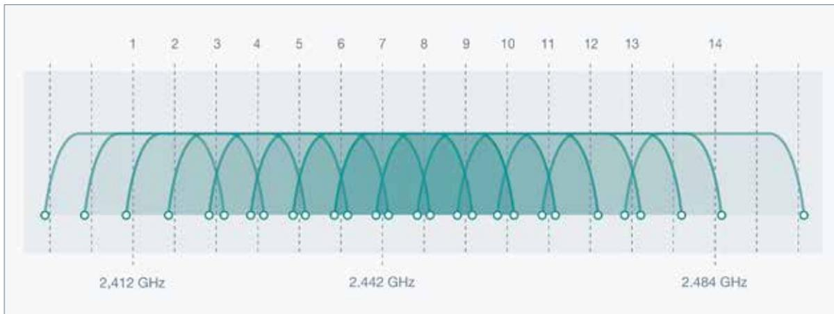
Figure 24: Channel designation in 2.4GHz band according to IEEE 802.11
