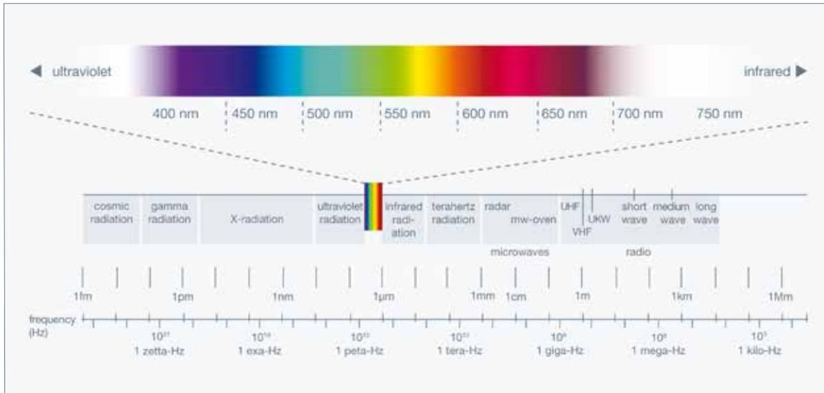
Figure 1: Electromagnetic spectrum
