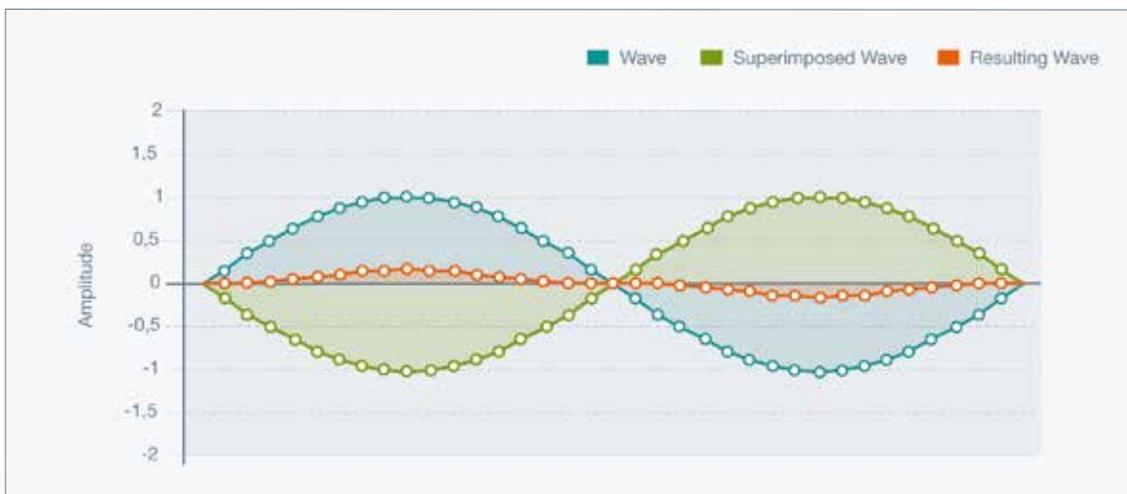
Figure 8: Negatively superimposed wave, destructive interference
