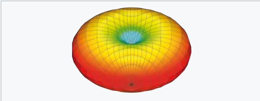
Figure 15: Radiation pattern of undisturbed dipole antenna
