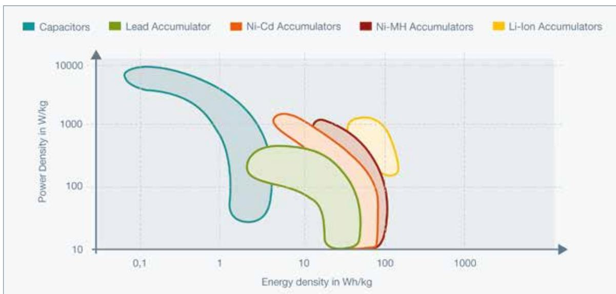
Figure 19: Power and energy density of different battery-types.
