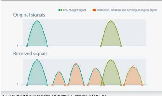
Figure 10: Receipt of the original signal and its reflections, bendings, and diffusions
