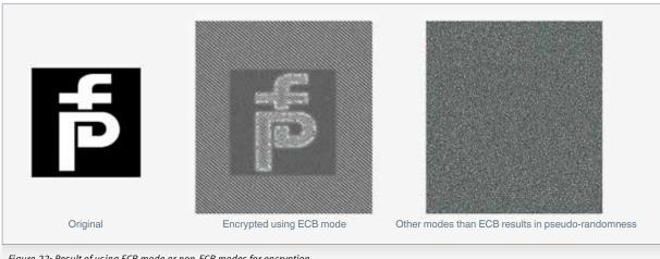
Figure 22: Result of using ECB mode or non-ECB modes for encryption
