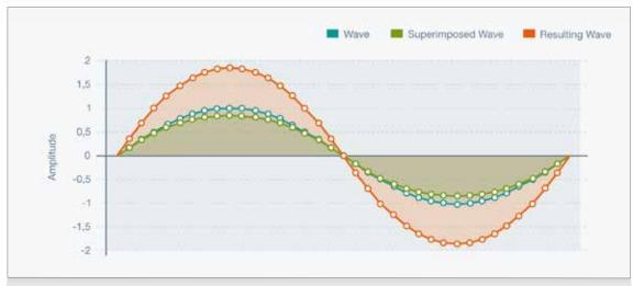
Figure 7: Positively superimposed wave, constructive interference
