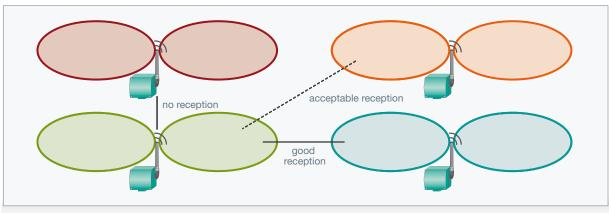
Figure 17: Reception quality depending on radiation pattern and relative position of radios
