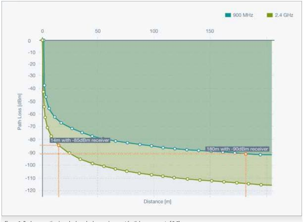
Figure 5: Real propagation in a shadowed urban environment (path loss exponent of 3.7)
