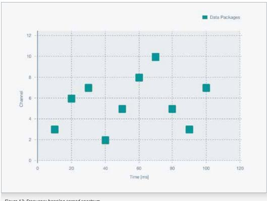
Figure 13: Frequency hopping spread spectrum
