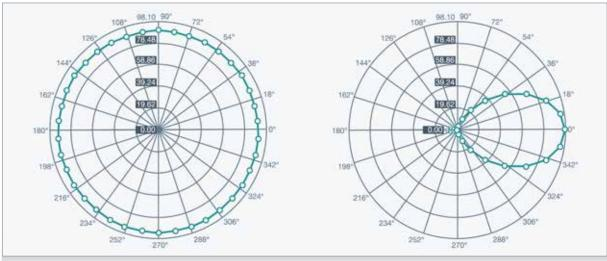
Figure 18: Radiation pattern of omnidirectional and directional antennas
