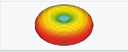
Figure 15: Radiation pattern of undisturbed dipole antenna
