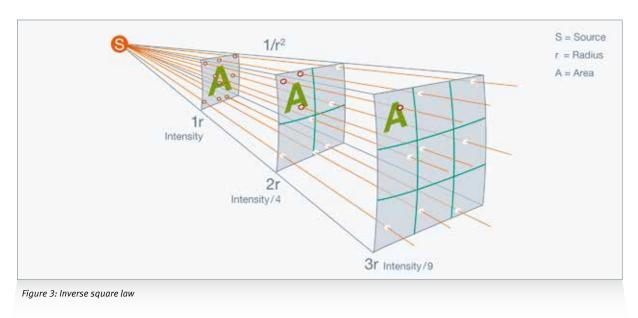
The result is that, with increasing distance, the density of the signal decreases with the function  $1/r^2$ . When doubling the distance, the signal density is just 1/4, with tripling the distance the signal density is 1/9.
