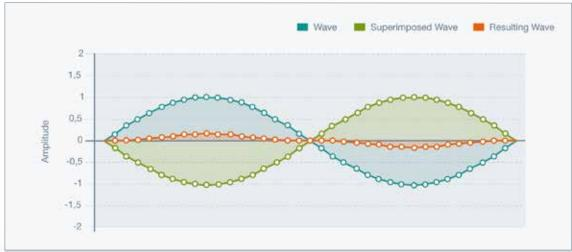
Figure 8: Negatively superimposed wave, destructive interference
