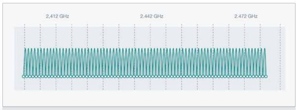
Figure 25: Channel designation in 2.4GHz band according to IEEE 802.15.1
