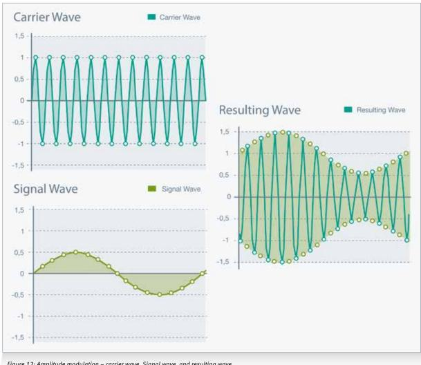
Figure 12: Amplitude modulation – carrier wave, Signal wave, and resulting wave
