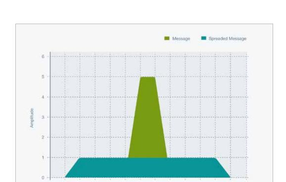
Figure 14: Direct sequence spread spectrum
