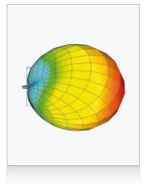
Figure 16: Radiation pattern of dipole with reflective plane in different distances
