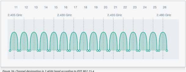
Figure 26: Channel designation in 2.4GHz band according to IEEE 802.15.4
