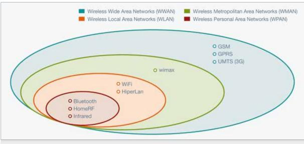
Figure 27: Standards for WPAN, WLAN, WMAN, and WWAN
