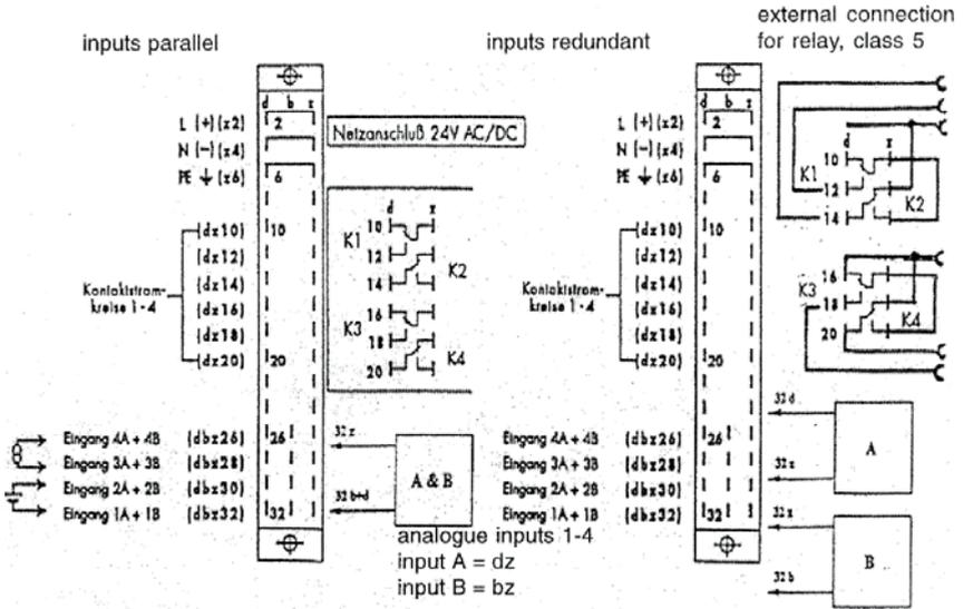
Connectors illustrated bridged are connected internal multi-pole connectors as per DIN 41 612, series F
