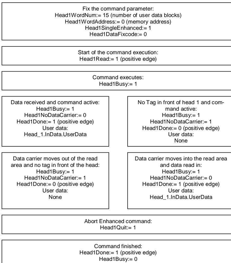
Single Write Words: (head 1; 15 data blocks starting at address 0)
