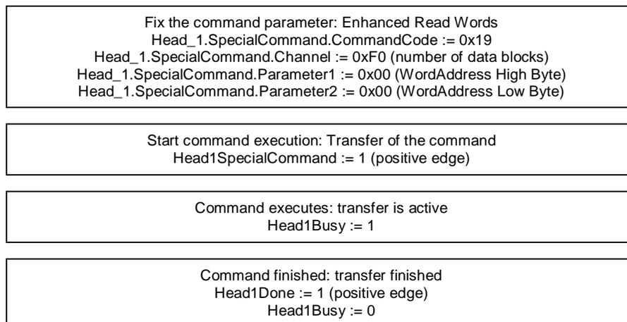
The number of the performed commands inside the command list is 10. The parameterization of the command list is finished by closing of the command list.
