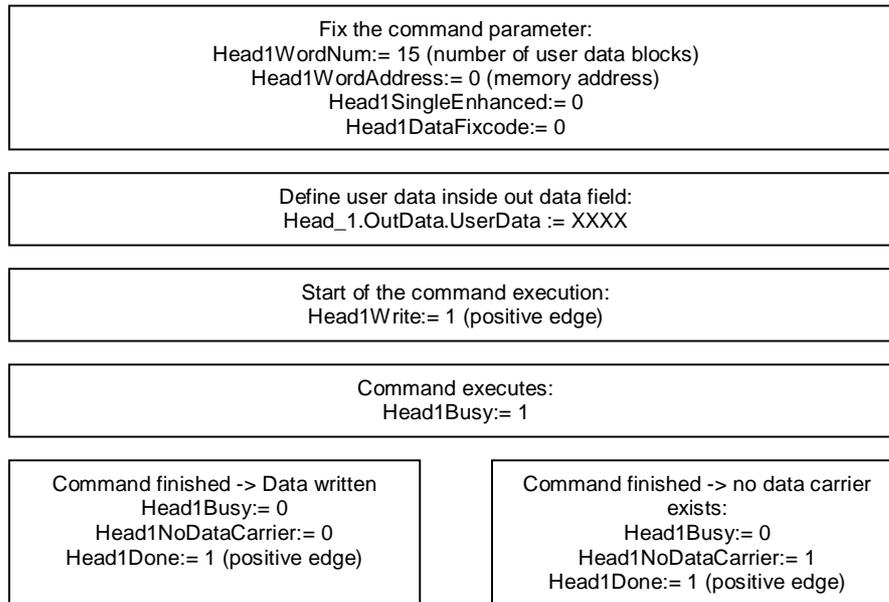
Enhanced Write Words: (head 1; 15 data blocks starting at address 0)
