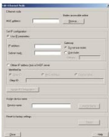
In this window you can with “Browse” search for all connected Profinet-IO nodes. Afterwards you can execute a new parameterization for the IP-Address and the Profinet-IO name.
