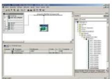
Per double click on the symbol of the IDENTControl a window with the properties of the Profinet-IO node will open. Now you are able to reconfigure the name of the Profinet-IO node (here: identcontrol).
