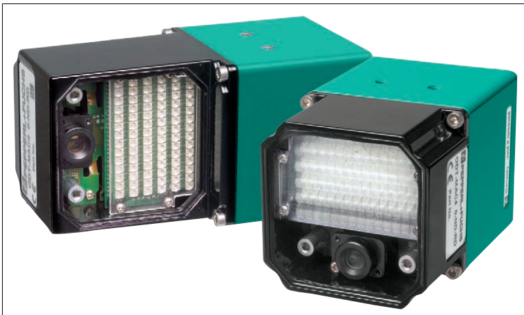
Figure 4.1 The two housing designs of the stationary read device: straight and angled
