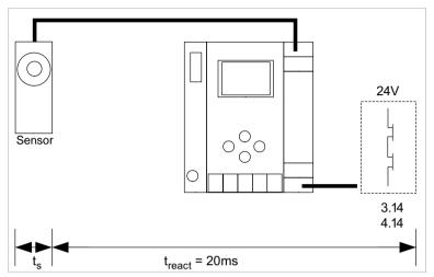
$t_s$  = maximal reaction time of the sensor (see data sheet)
