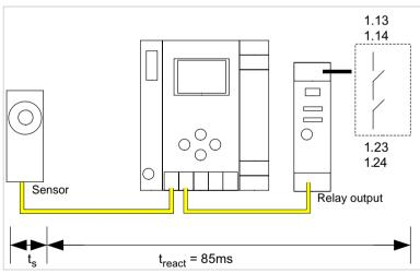
$t_s$  = maximal reaction time of the sensor (see data sheet)  $t_{react}$  = maximal system reaction time
