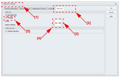
Here the group and device addresses are assigned and the safe programs for the individual Gateways managed. Information about the IP addresses of the participating devices are also stored in the project structure.
