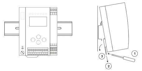
To remove, press the holding clamps [2] down using a screwdriver [1], press the unit firmly against the upper rail guide and lift out.
