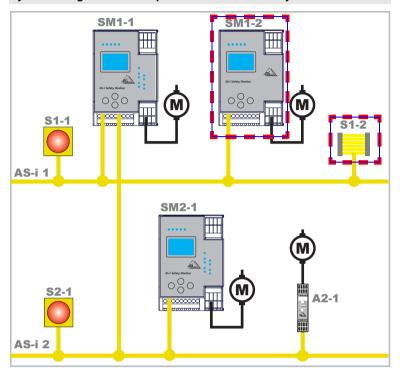
Upon activation of safety light barrier S1-2, the relay safety output of safety monitor SM1-2 is controlled.
