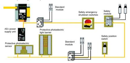
Fig. 4-1. Safe and standard components in an AS-i network
