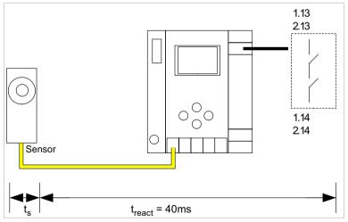
$t_{\rm S}$  = maximal reaction time of the sensor (see data sheet)  $t_{\rm react}$  = maximal system reaction time
