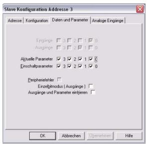
This window enables the user to edit a slave address and to set AS-i parameters or AS-i configuration data. Additionally, inputs and outputs can be tested.
