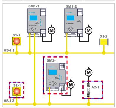
Upon locking of the EMERGENCY-OFF switch S2-1, the motor starter is controlled via the safe AS-interface output of safety monitor SM2-1.
