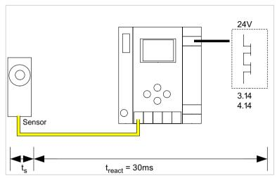
$t_s$  = maximal reaction time of the sensor (see data sheet)  $t_{treact}$  = maximal system reaction time
