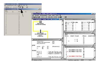
Configuring the AS-i network is easily accomplished by first connecting each AS-i slave separately to the AS-i line and setting its address, followed by pressing the button "Store configuration" to store the existing AS-i network in the AS-i master as configuration data.
