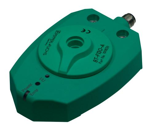
The PMI360DV-F130-IU-V15 has an analog output for the analog indication of angular positions. For high resistance loads (>3.3 k $\Omega$ ), the angular position is output as a voltage value 0 ... 10 V DC and for low resistance loads (<400  $\Omega$ ), as a current value 4 ... 20 mA.
