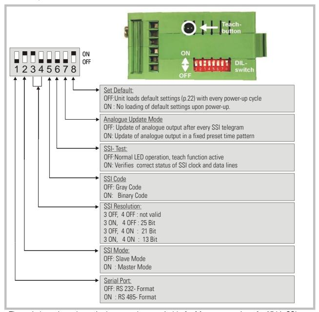
The switch settings shown in the example are suitable for Master operation of a 25 bit SSI encoder with Gray coded output.
