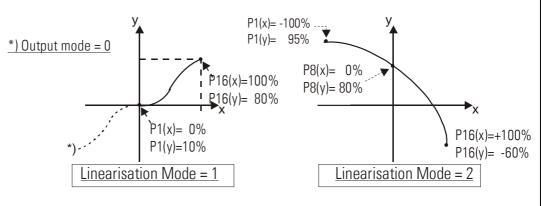
You can visualize your curve on the PC screen or by means of the internal PC scope or any external oscilloscope. For this, select TOOLS, then TEST and there "Analogue Voltage Function". The unit will now simulate a repeating motion of the encoder over the full range and generate the analogue signal accordingly. When you use the Scope function of the operator software, you must set the serial code " :1" to record the analogue output.
